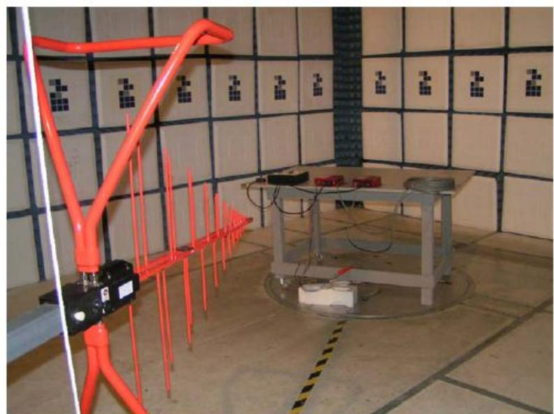
**Radiated Emission Test Set-up Back View**
