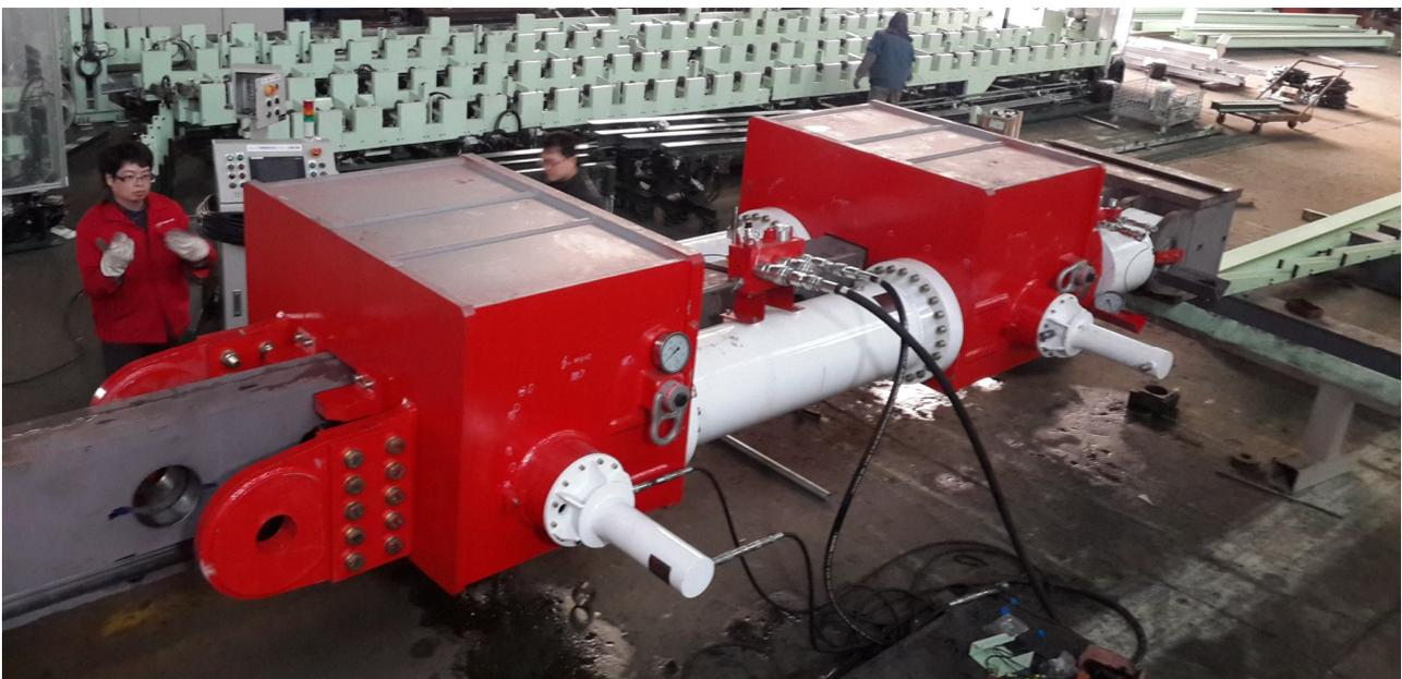
DL-CP600 pinned climbing jack load testing
