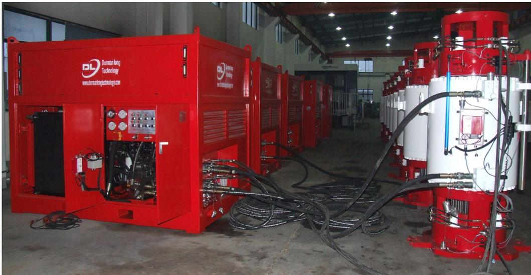
DL-L120/2/300/D Diesel powered hydraulic power packs
